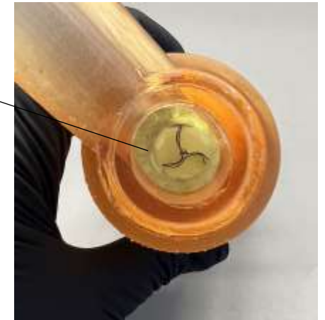
Valve viewing window
